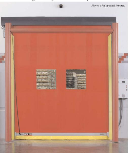
**Self-Repairing** – If the door is impacted from either direction, a pre-programmed, self-repairing feature automatically brings the door to the full open position where it is reset. The software then initiates the closing cycle – without user intervention.
